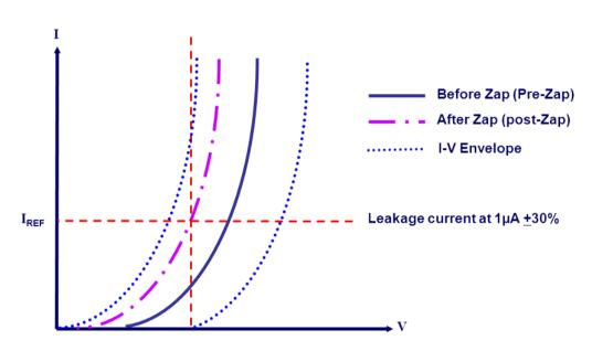
Pass/Fail Criteria: Variation of Leakage Current and I-V Shift in Pre-Zap and Post-Zap curves
