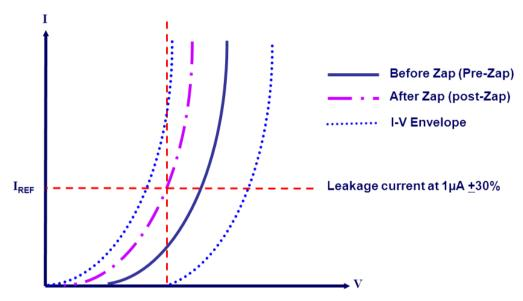
Pass/Fail Criteria: Variation of Leakage Current and I-V Shift in Pre-Zap and Post-Zap curves
